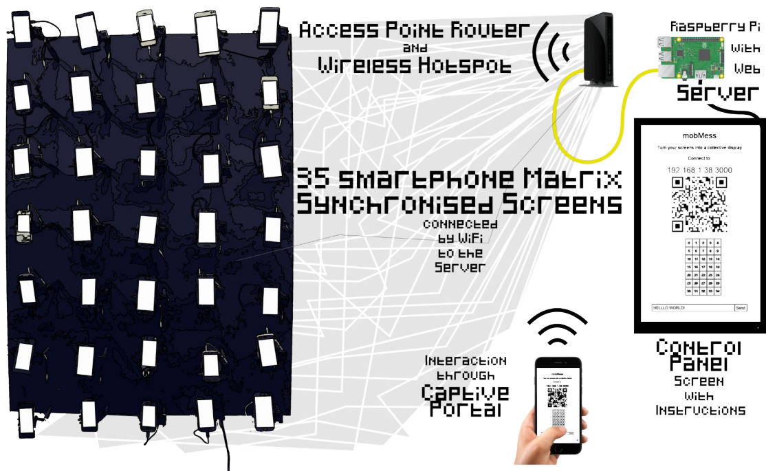
Figure 49: mobMess installation diagram.
